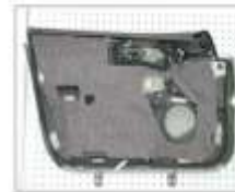
Door trim base material that uses kenaf
