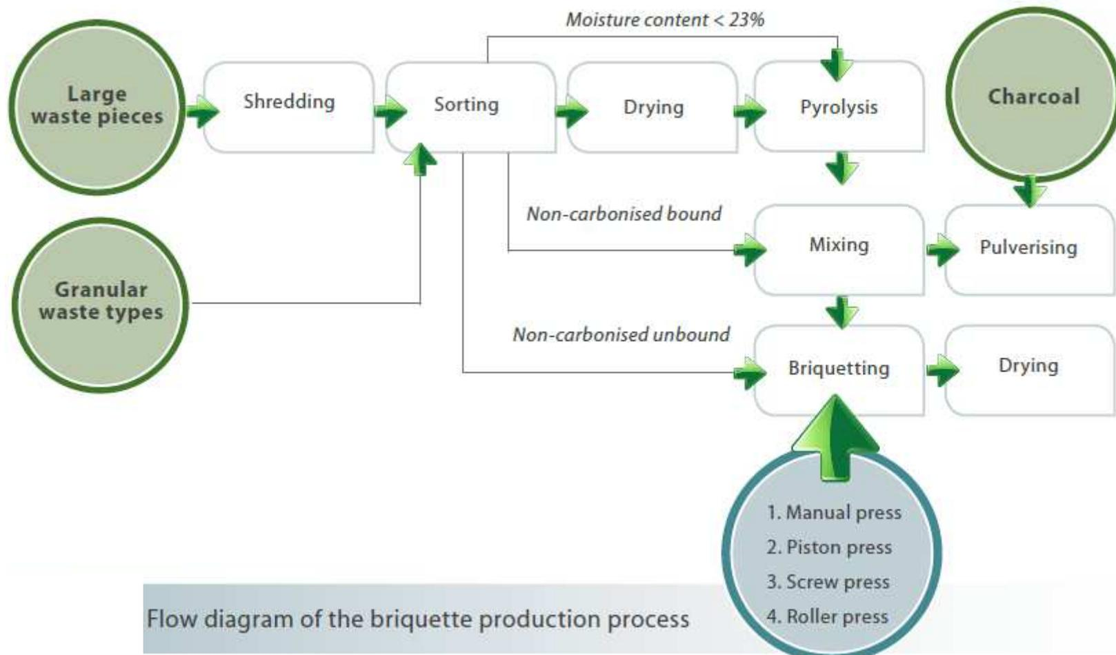
Flow diagram of the briquette production process
